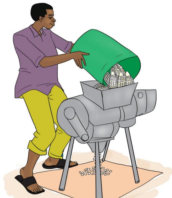
Motorized mechanical sheller
